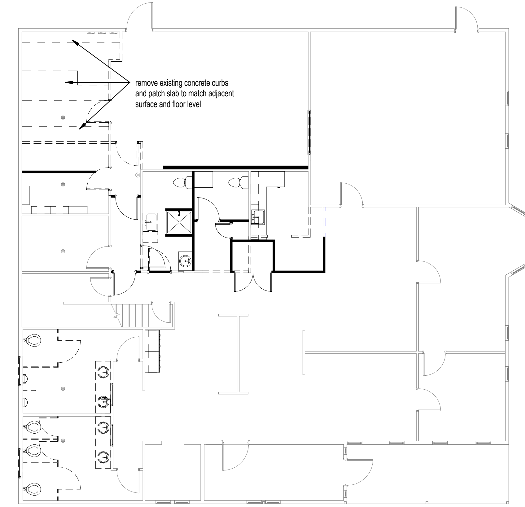
2 FIRST FLOOR DEMOLITION & NEW WALL PLAN 1/8" = 1'-0"
