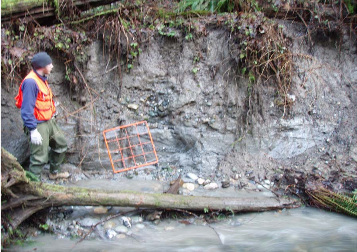
Photo 13. Typical exposed bank. Material is mainly silty clay with lenses of gravel and scattered cobbles.
