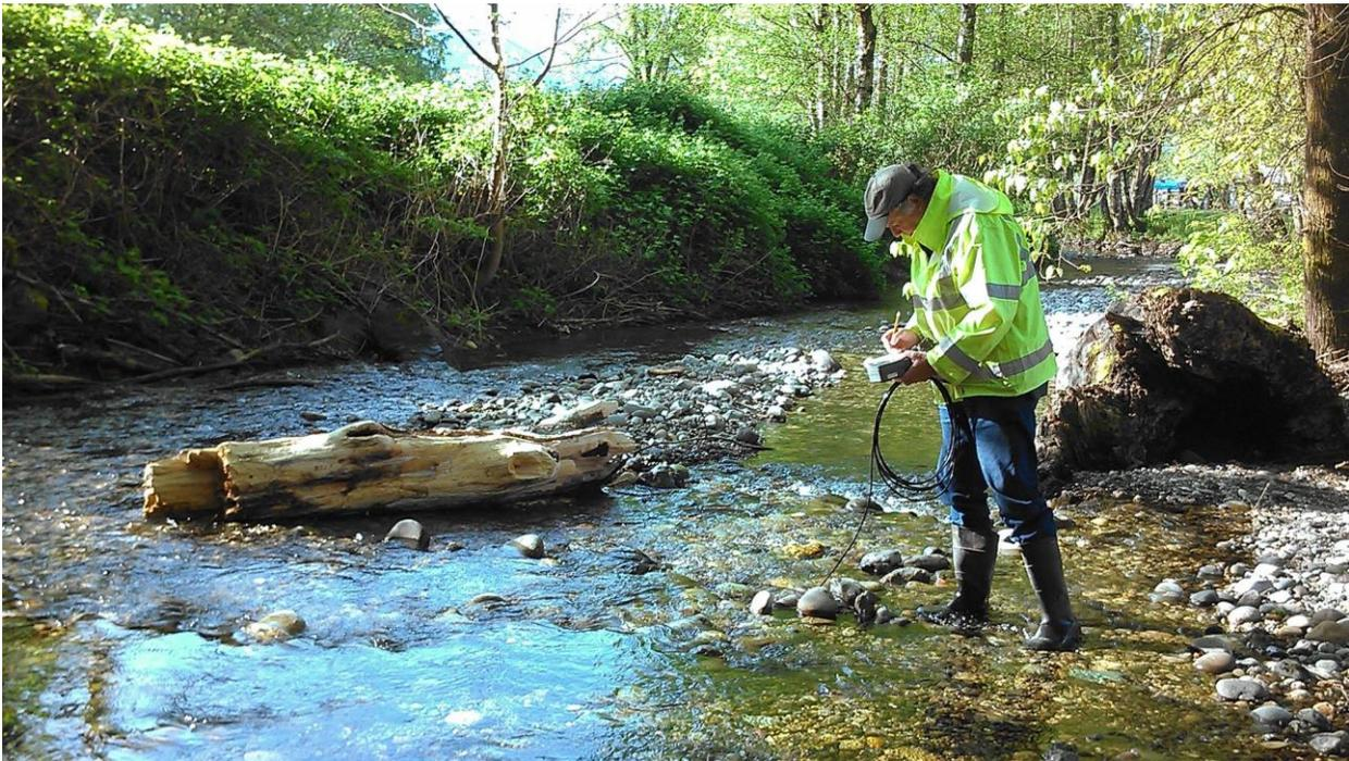
**Figure 2. Taking dissolved oxygen readings at Red Cabin Creek**
