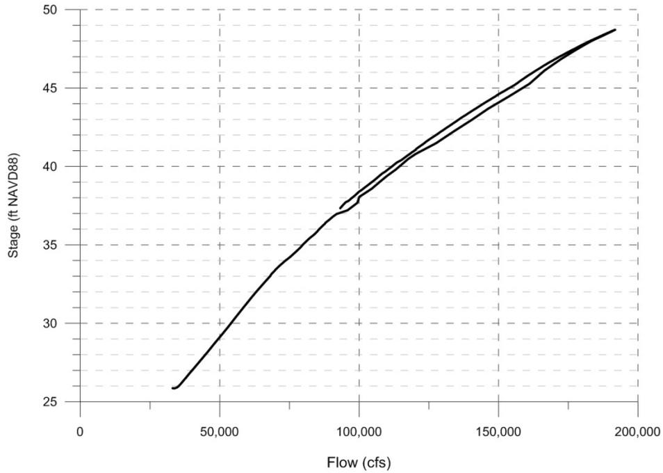
Existing Condition (No Breach) Rating Curve
