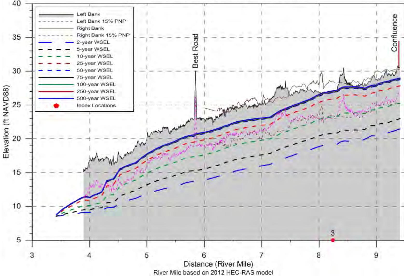
Existing Condition (No Breach) Rating Curve
