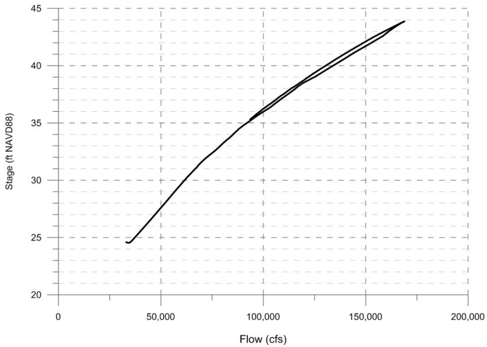
Existing Condition (No Breach) Rating Curve
