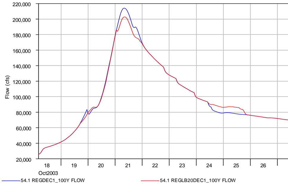
**Figure 4-11: 100-year hydrographs, Skagit River near Concrete, for 1 December for existing regulation at Upper Baker and Ross Dams, with (red line) and without (blue line) flood control storage at Lower Baker.**
