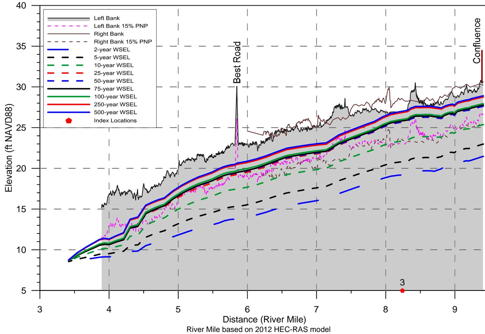
Note: Bank elevation profiles represent the "with alternative" condition.
