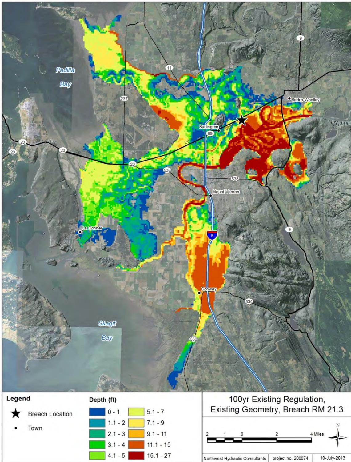
**Figure 5-3: Maximum flood depths for 100-year event under existing conditions with levee breach at RM 21.3**
