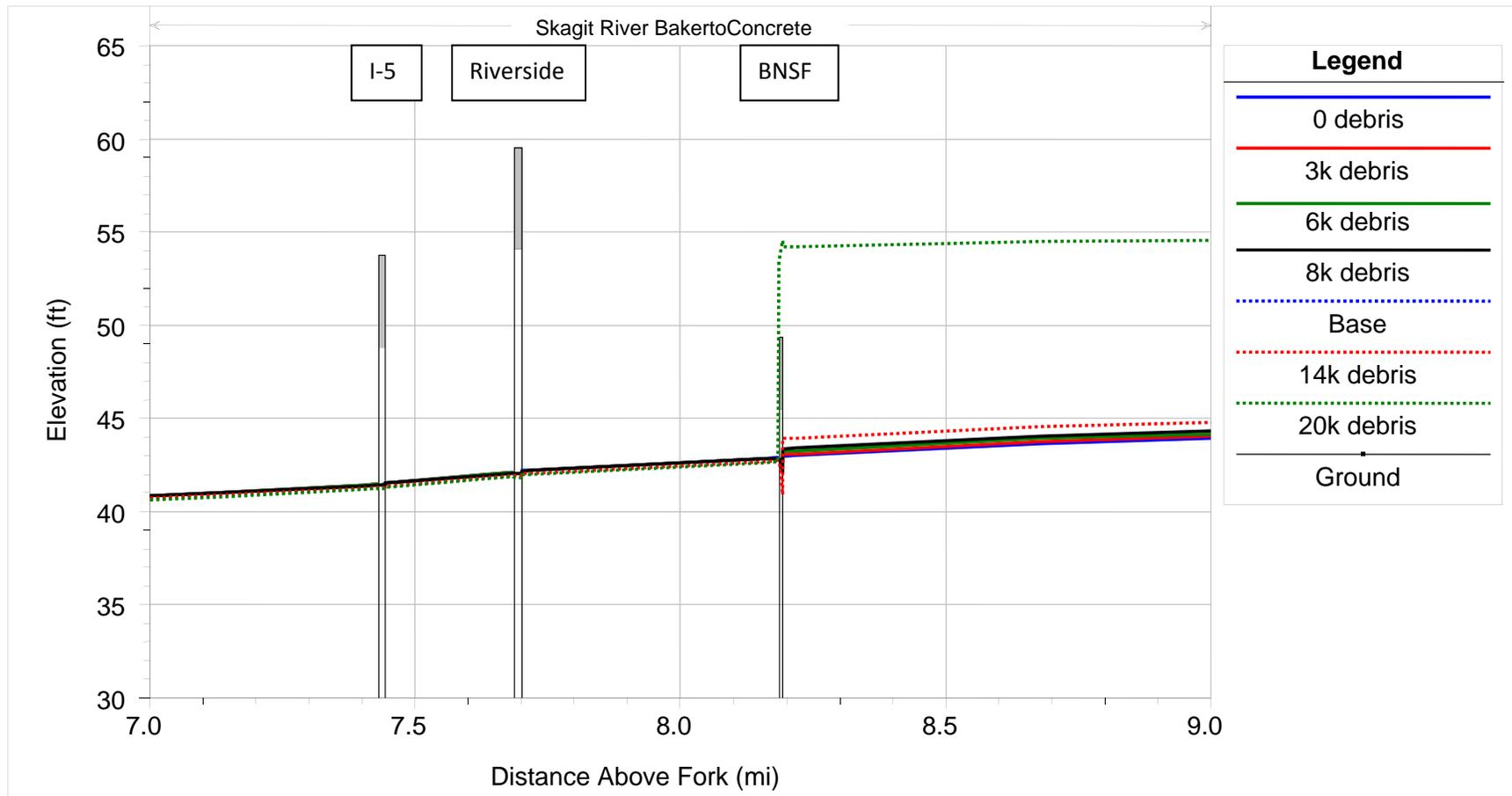
**Figure 2-13: 150,000 cfs Water Surface Profiles – Debris Sensitivity.**
