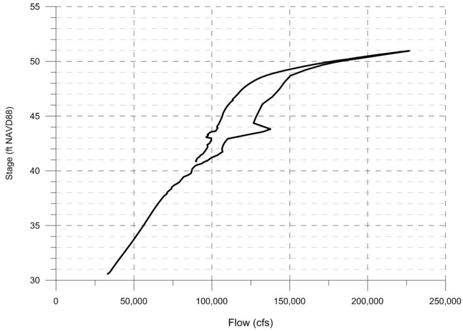
Existing Condition (No Breach) Rating Curve
