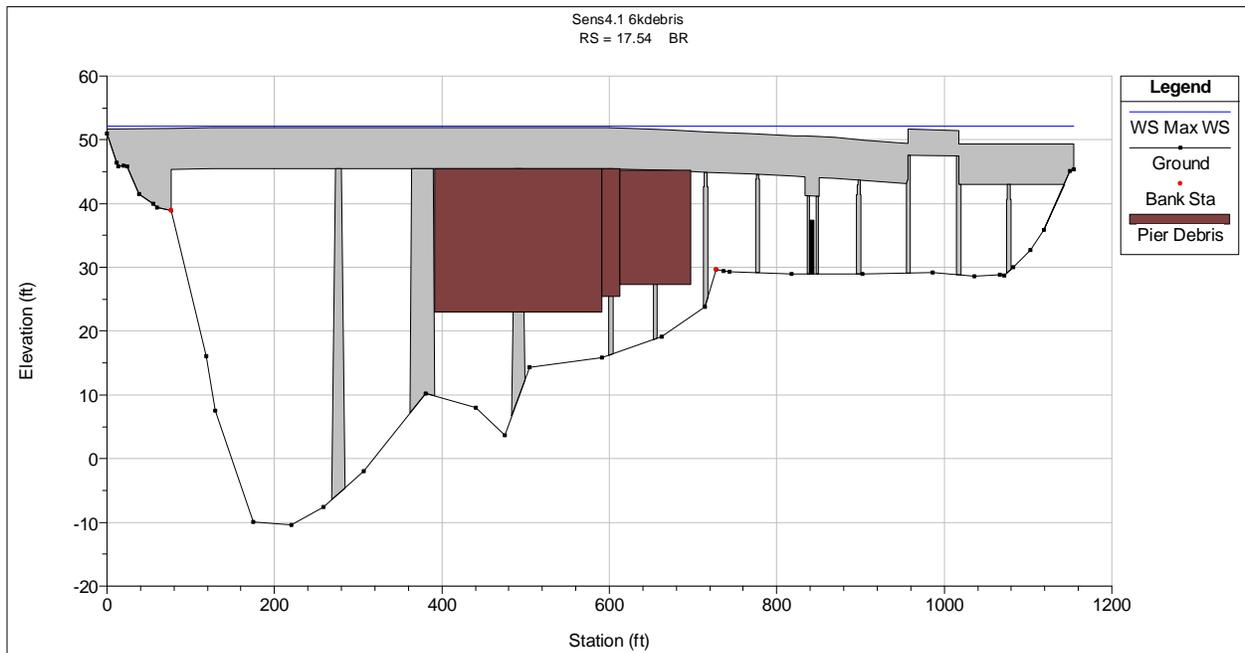
Figure 2-7: BNSF Bridge – 6,000 sq. ft. of debris.
