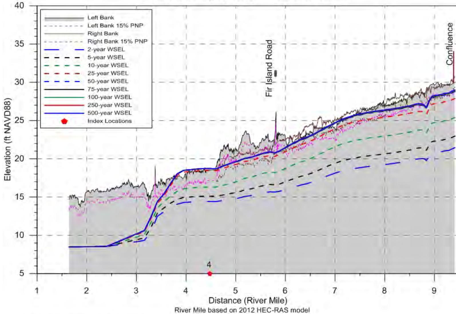
Note: Bank profiles and PNPs reflect improved levee ("baseline") condition
