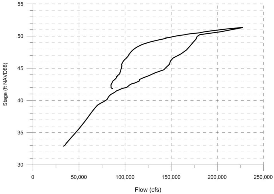
Existing Condition (No Breach) Rating Curve
