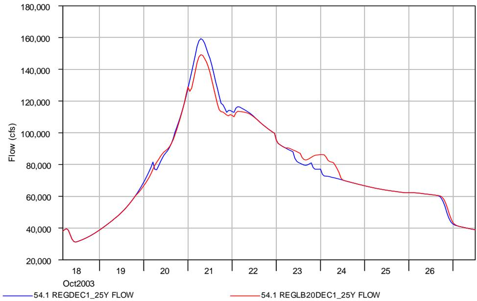
**Figure 4-10: 25-year hydrographs, Skagit River near Concrete, for 1 December for existing regulation at Upper Baker and Ross Dams, with (red line) and without (blue line) flood control storage at Lower Baker.**
