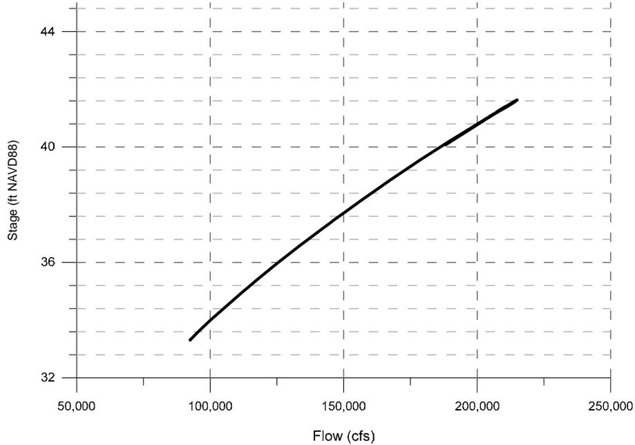
Note: Rating curve reflects hydraulic conditions post activation of the "fuse plug"
