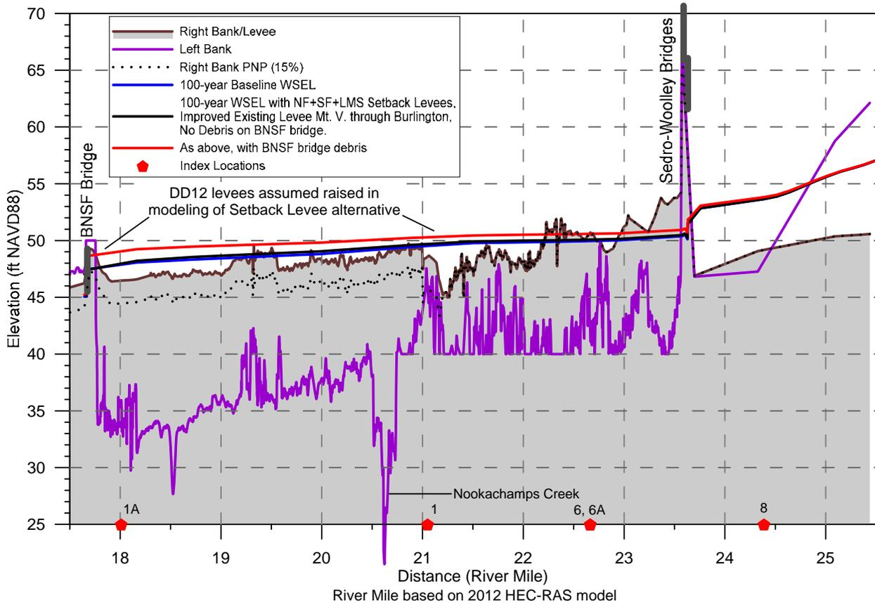
Note: Levee elevations and PNP profiles represent the improved levee "baseline" condition.
