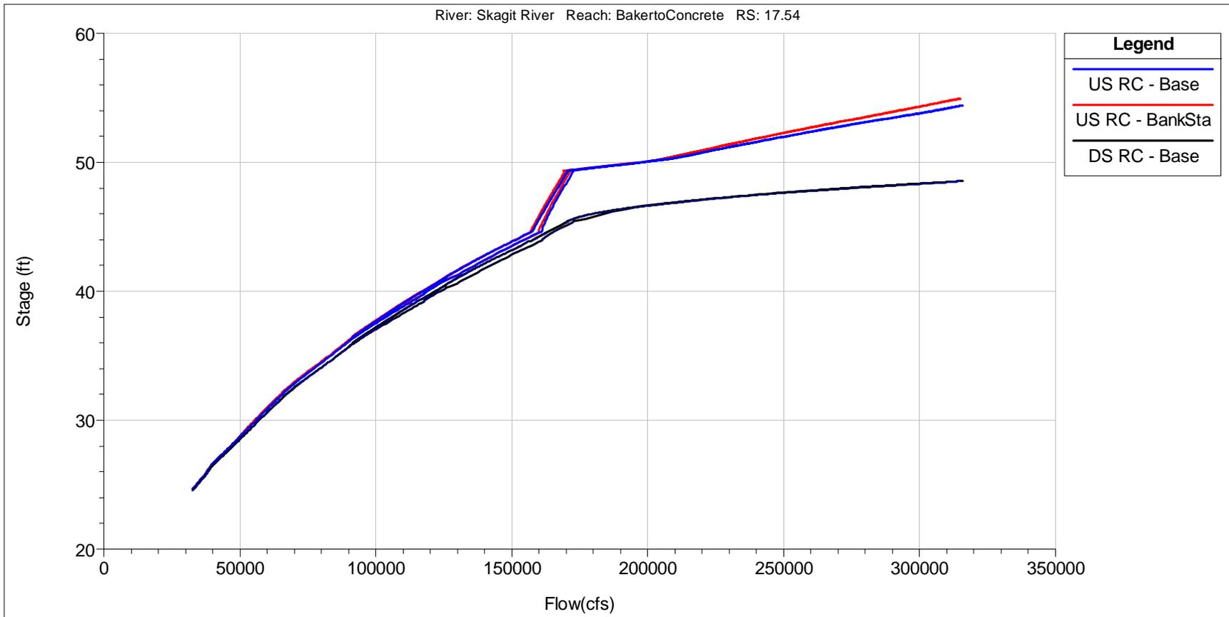
**Figure 2-18: BNSF Bridge Rating Curves – Bank Station Sensitivity.**
