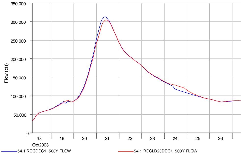
**Figure 4-12: 500-year hydrographs, Skagit River near Concrete, for 1 December for existing regulation at Upper Baker and Ross Dams, with (red line) and without (blue line) flood control storage at Lower Baker.**
