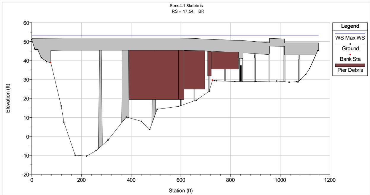
**Figure 2-8: BNSF Bridge – 8,000 sq. ft. of debris.**
