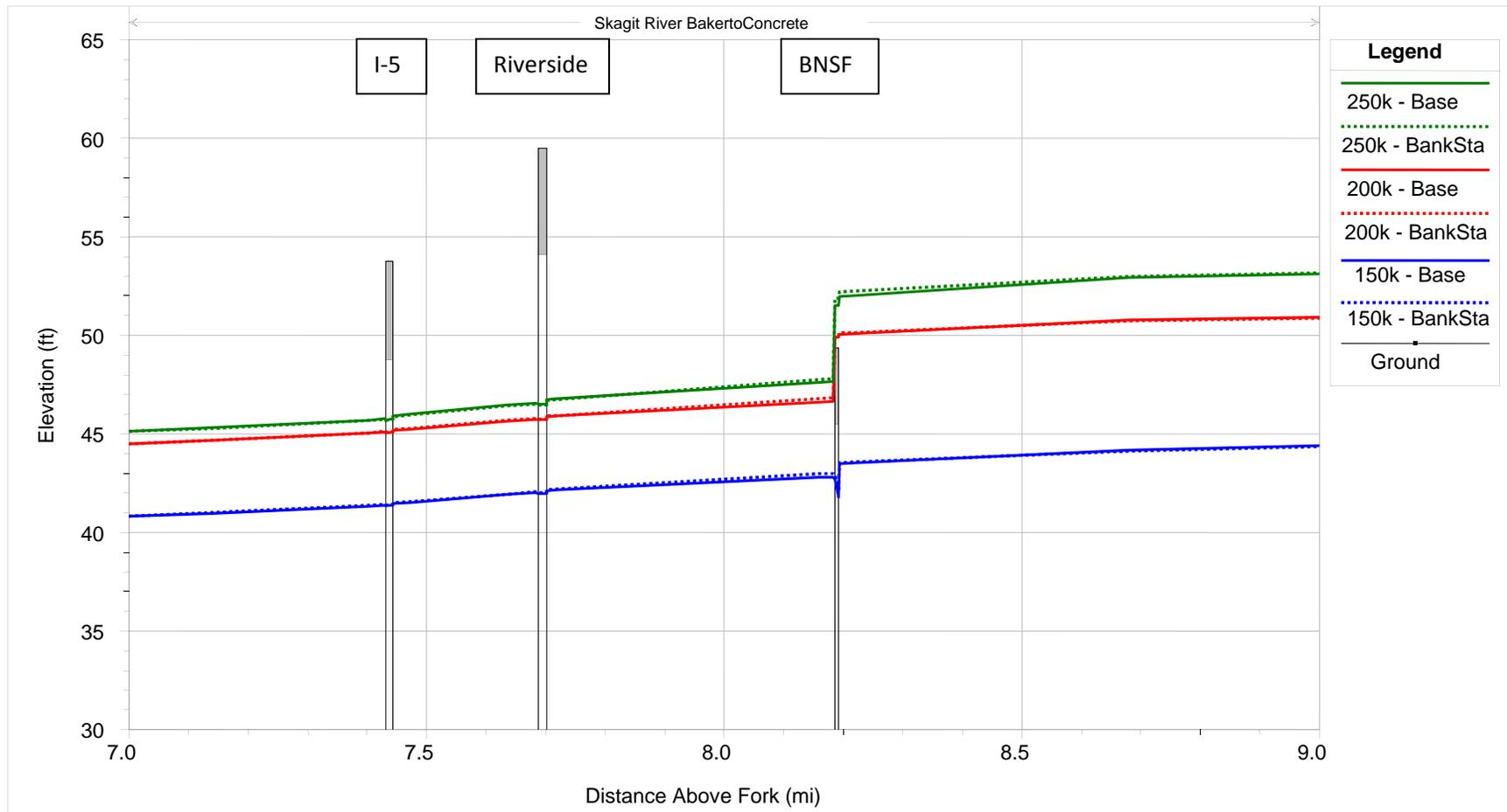
Notes: Base scenario with right bank station at edge of low flow channel. Simulations assume no scour.
