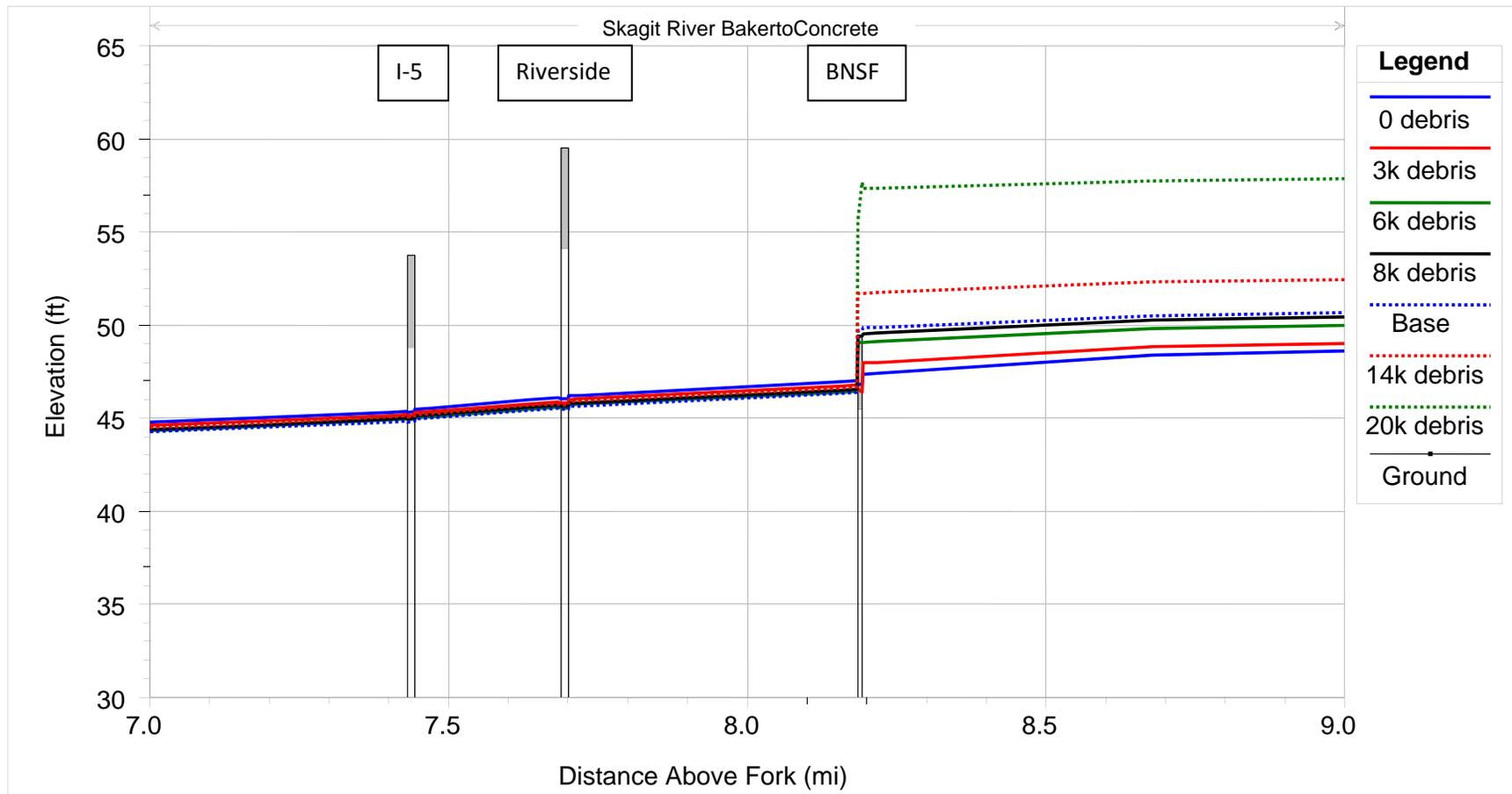
**Figure 2-14: 200,000 cfs Water Surface Profiles – Debris Sensitivity.**
