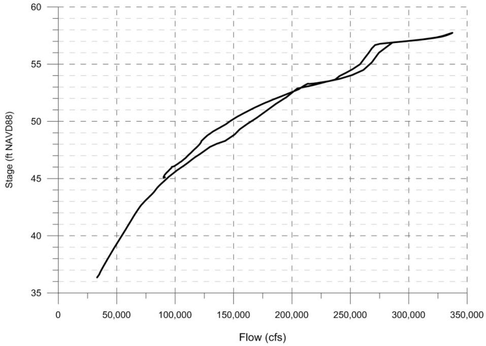
Existing Condition (No Breach) Rating Curve
