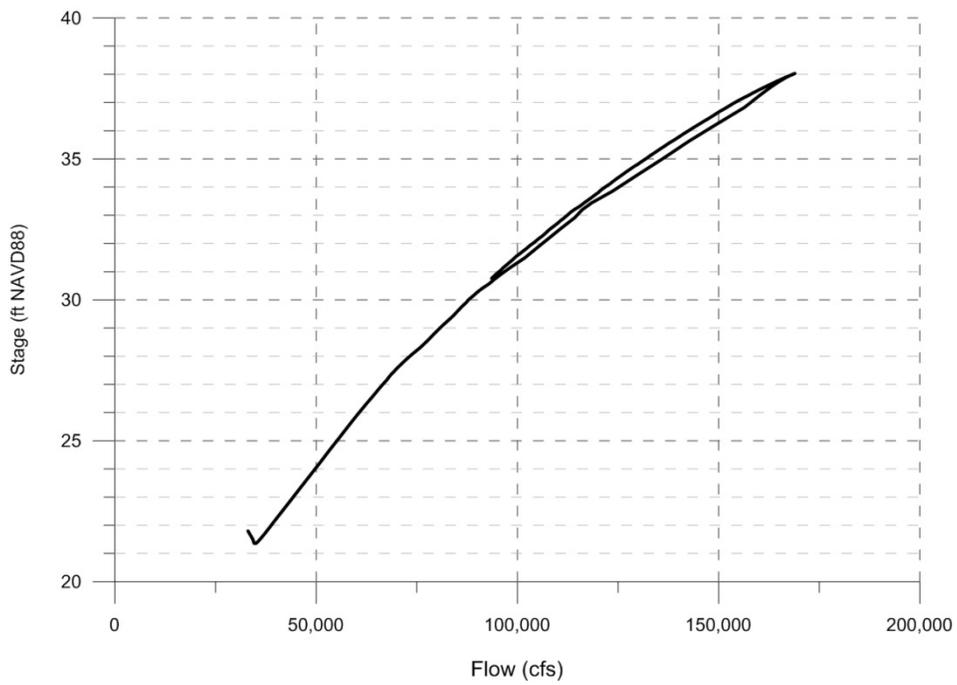
Existing Condition (No Breach) Rating Curve
