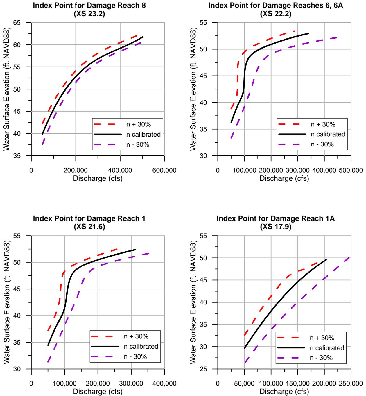
**Figure 5-10: Stage-discharge ratings with uncertainty in roughness, existing conditions**
