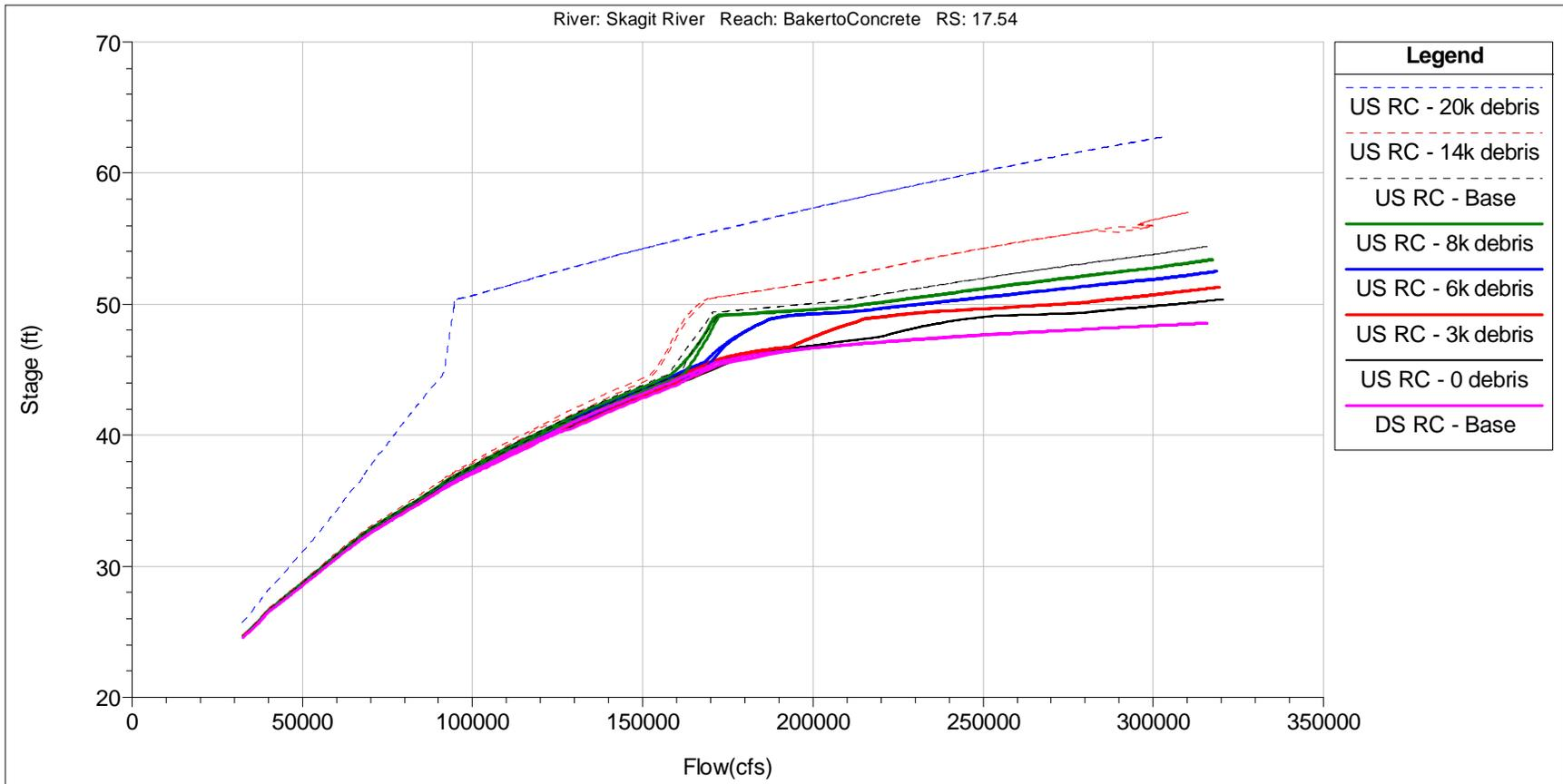
**Figure 2-12: BNSF Bridge Rating Curves – Debris Sensitivity.**
