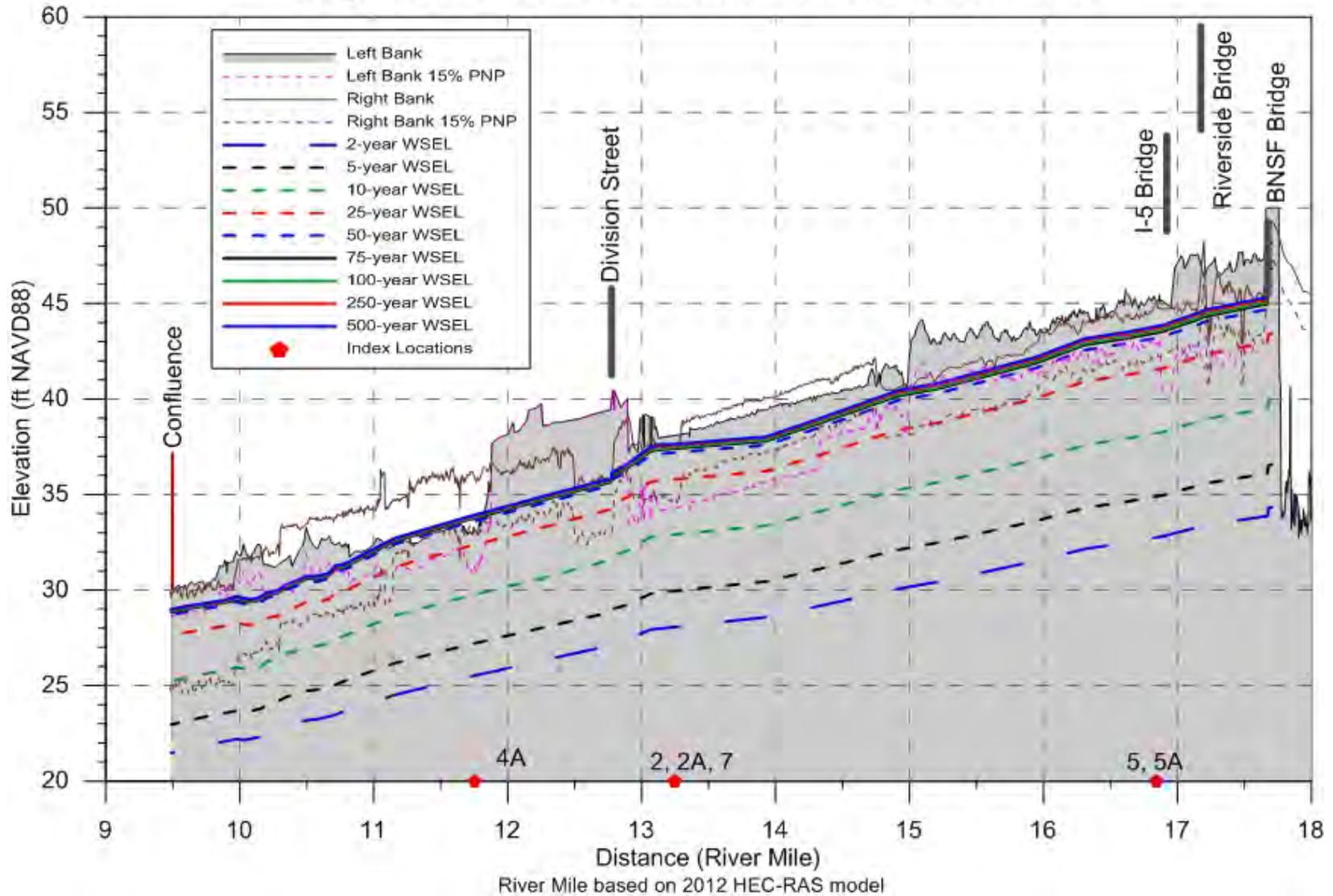
Existing Condition Geometry, No Breach
