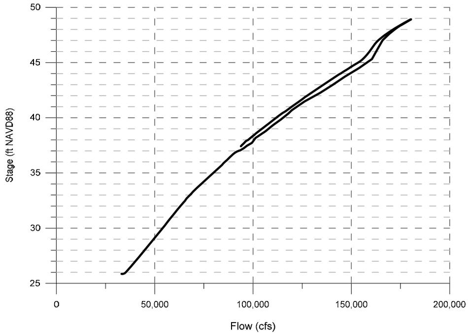
Baseline (Improved Levee) Condition, No Breach Rating Curve
