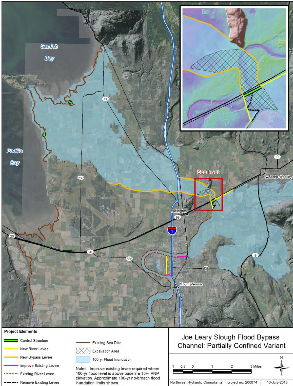
**Figure 6-9: Joe Leary Slough Flood Bypass: Partially Confined Variant**
