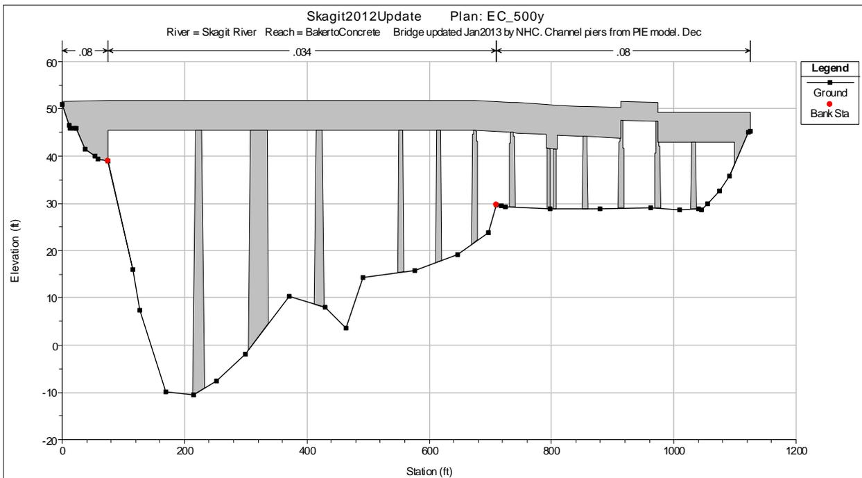
Figure 2-23: Final BNSF bridge geometry after January 2013 refinements
