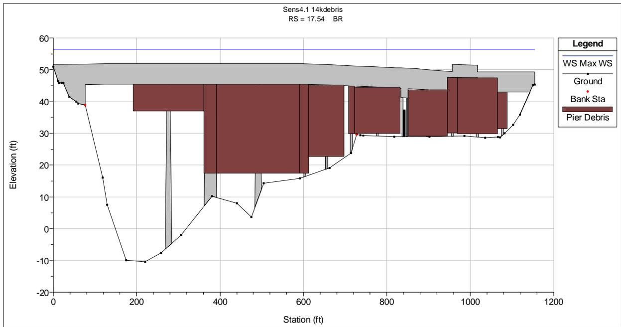
**Figure 2-10: BNSF Bridge – 14,000 sq. ft. of debris.**
