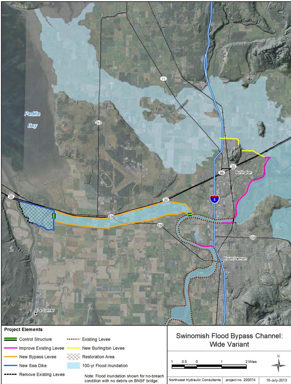
**Figure 6-16: Swinomish Flood Bypass: Wide Confinement Variant**
