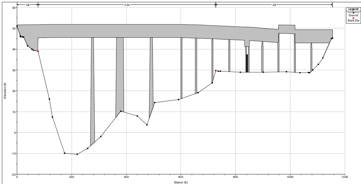
**Figure 2-2: BNSF bridge geometry from November 2012 survey.**
