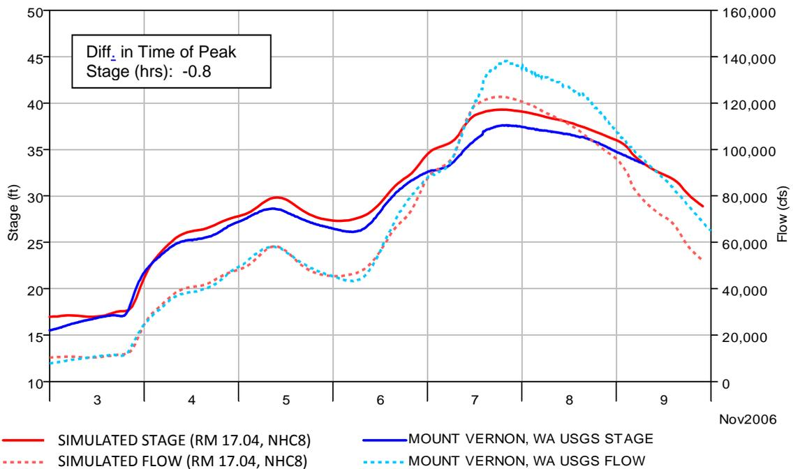
**Figure 7. Comparison of USGS Gage Record to HEC-RAS Simulated Stage and Discharge Hydrographs at Mount Vernon for November 2006 Event**
