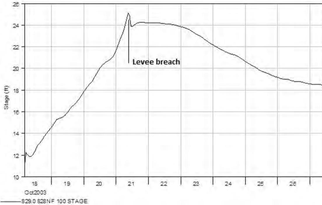
**Figure 5-2: Existing Condition 100-Year With-Breach Stage Hydrograph, North Fork XS 829.**
