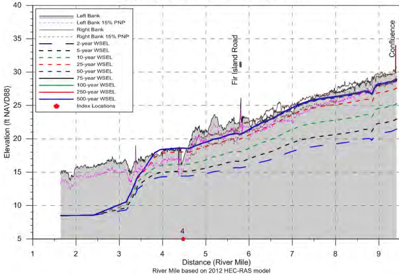
Existing Condition Geometry, No Breach
