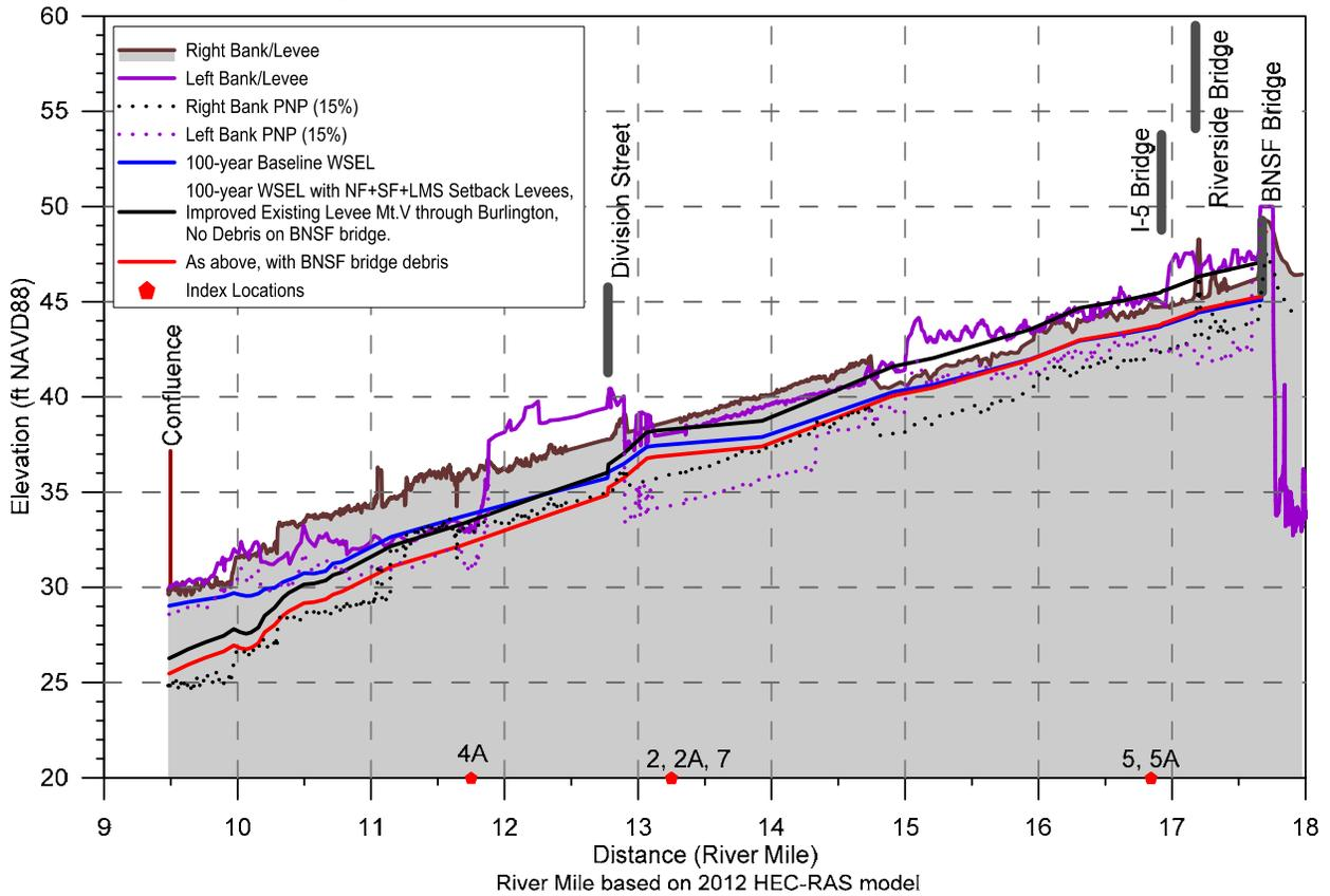
Note: Levee elevations and PNP profiles represent the improved levee "baseline" condition.
