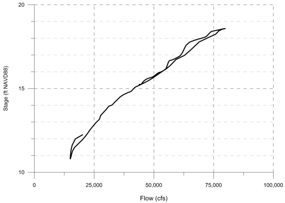
Existing Condition (No Breach) Rating Curve
