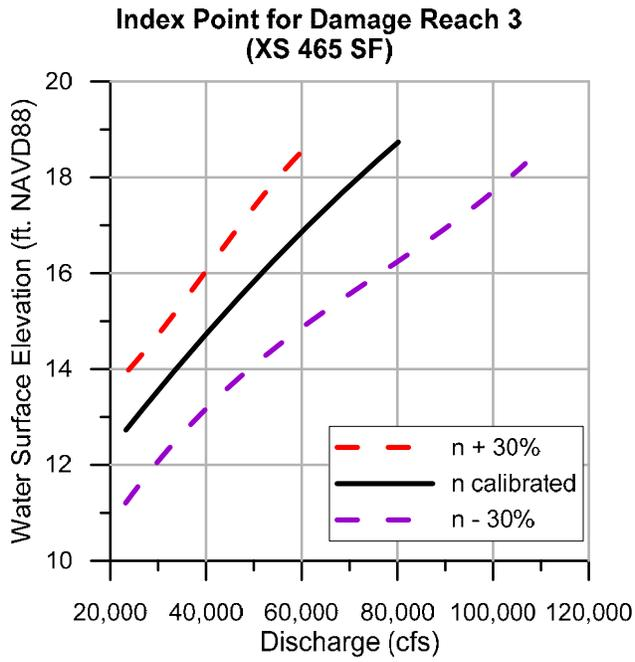
**Figure 5-10 (cont.): Stage-discharge ratings with uncertainty in roughness, existing conditions**
