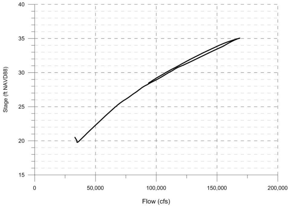
Existing Condition (No Breach) Rating Curve
