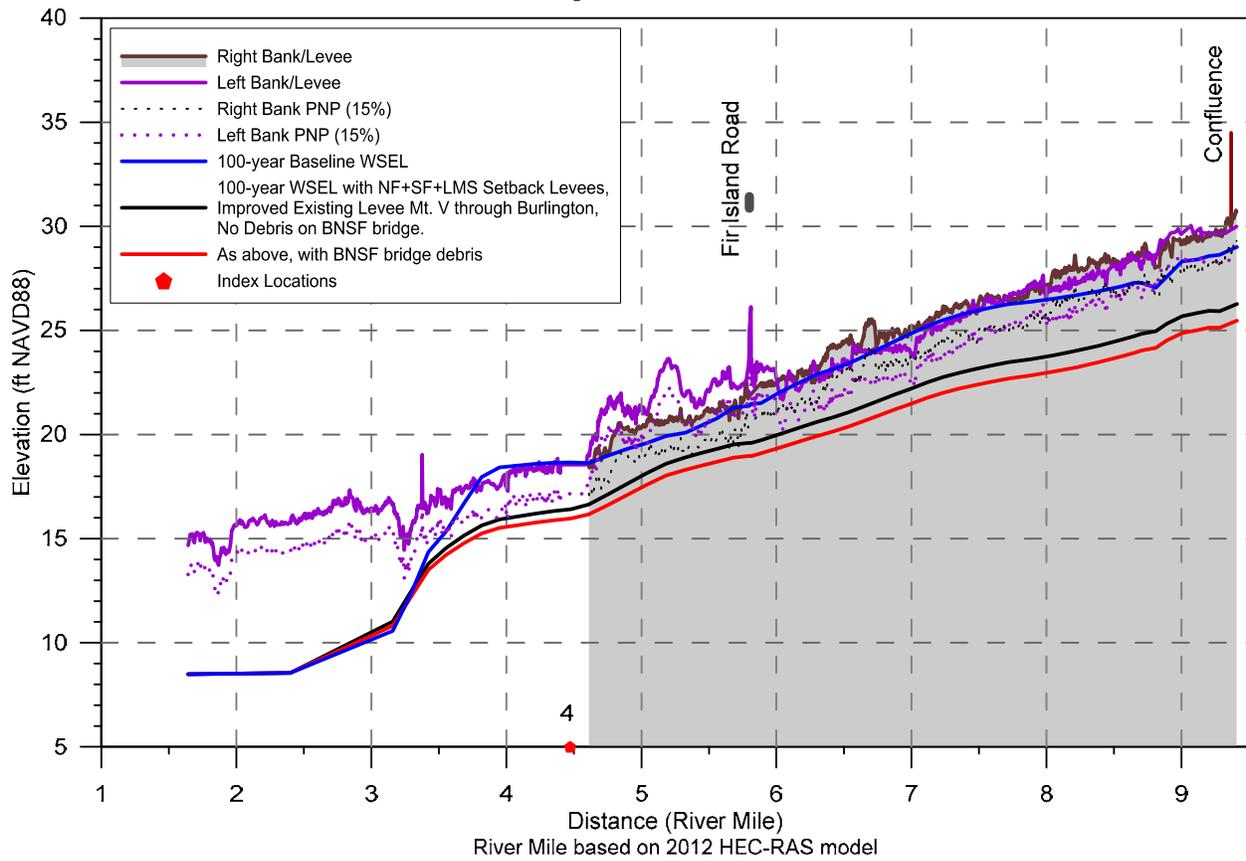
Note: Levee elevations and PNP profiles represent the improve levee "baseline" condition.
