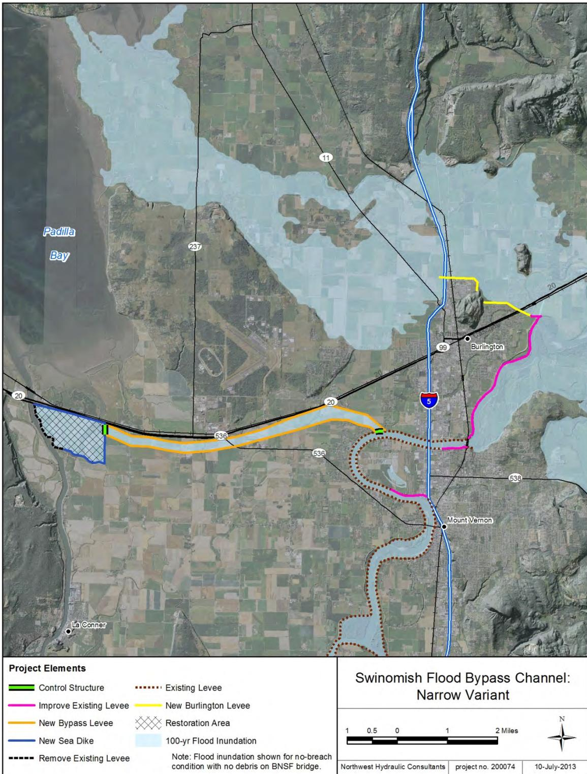
**Figure 6-17: Swinomish Flood Bypass: Narrow Confinement Variant**
