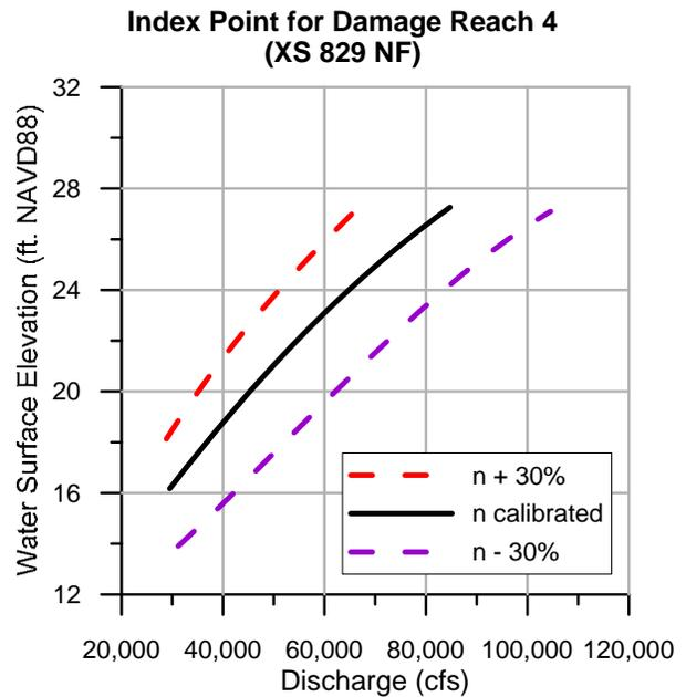
**Figure 5-10 (cont.): Stage-discharge ratings with uncertainty in roughness, existing conditions**
