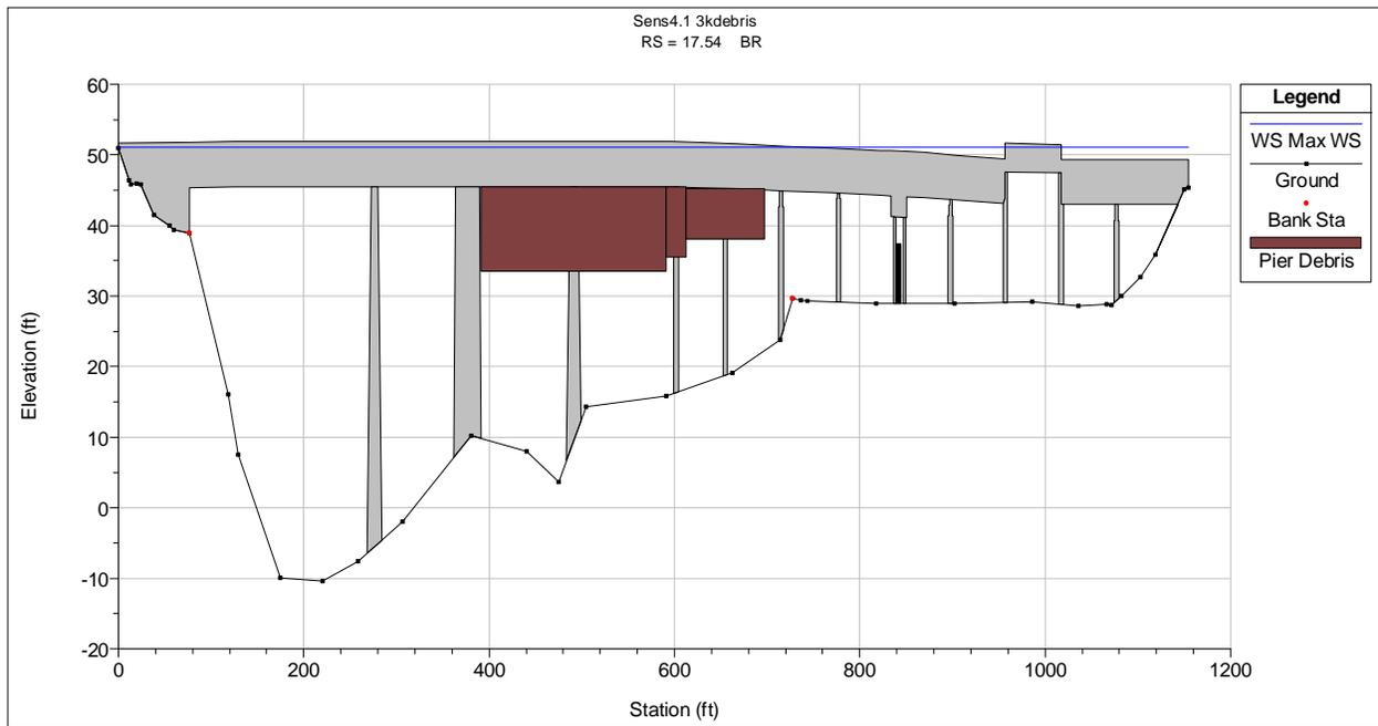
Figure 2-6: BNSF Bridge – 3,000 sq. ft. of debris.
