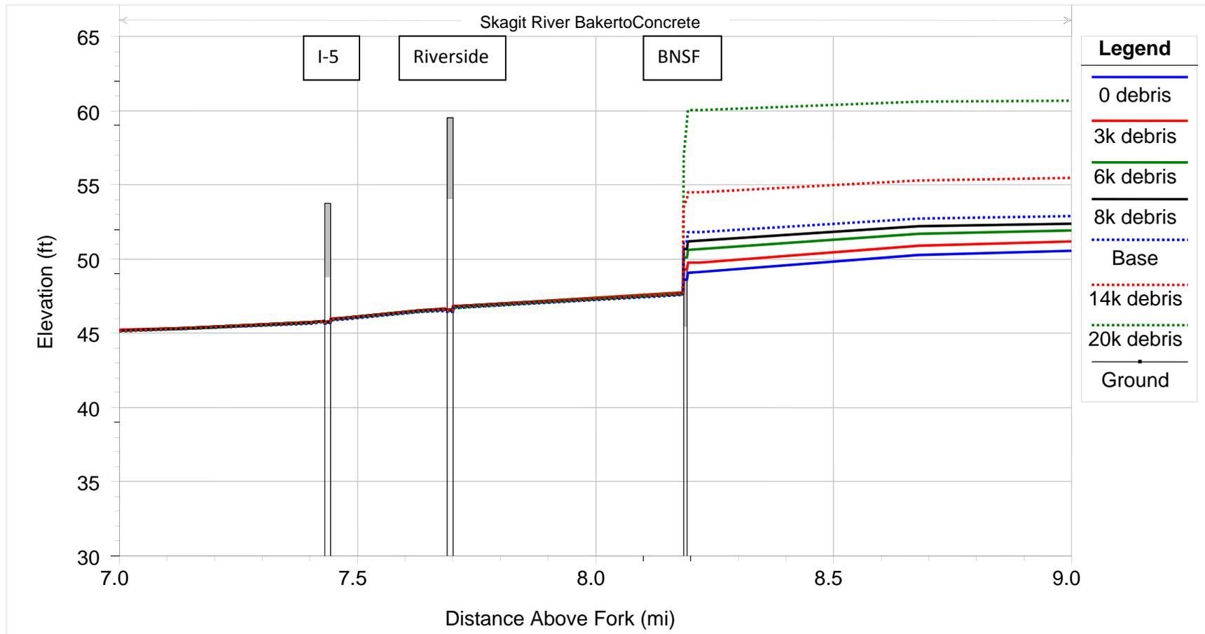
**Figure 2-15: 250,000 cfs Water Surface Profiles – Debris Sensitivity.**
