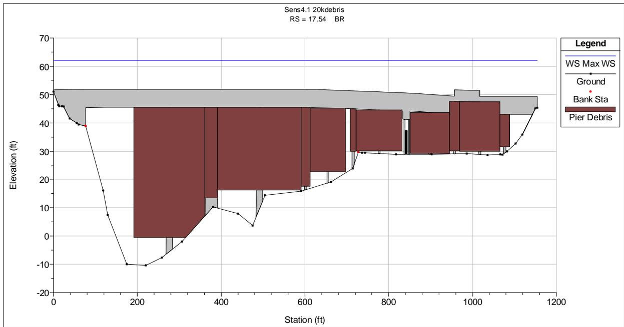
**Figure 2-11: BNSF Bridge – 20,000 sq. ft. debris.**
