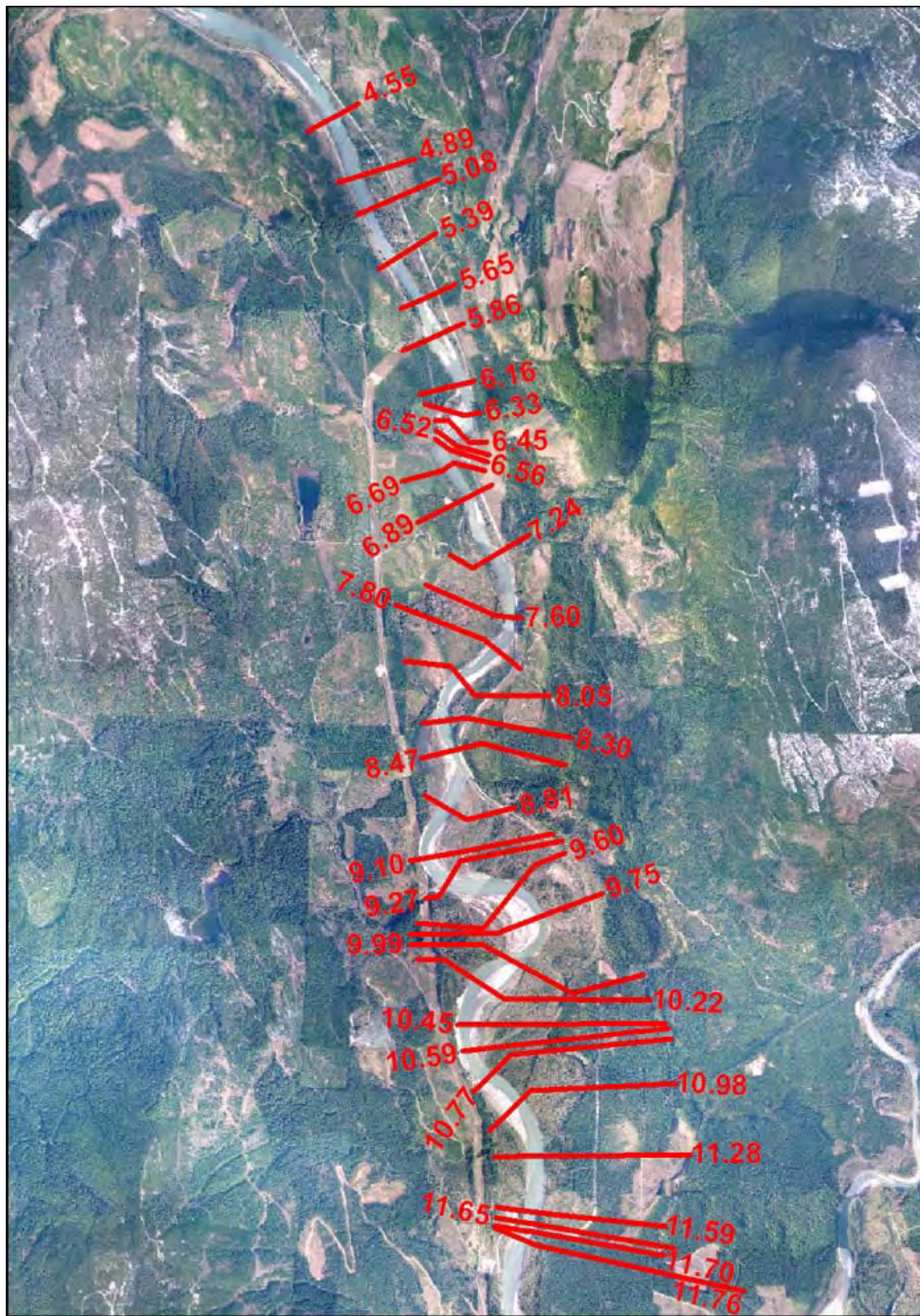
Figure 2. Location of HEC-RAS transects and corresponding analysis segments established to compare sediment transport, channel migration, and other analysis results.
