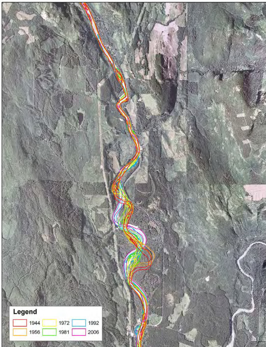
Figure 10. Locations of the main channel of the Sauk River in each set of aerial photographs analyzed for Phase 1. Mapped extent of side channels is indicated by shading.
