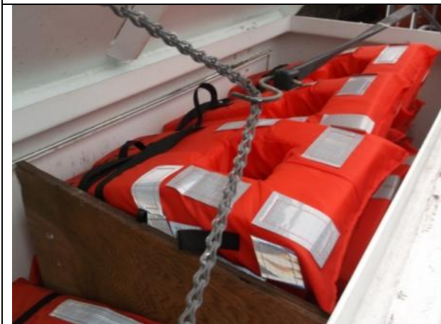
17 Typical Life Preserver Storage
