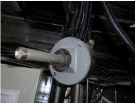
**17 Typical Engine Fire Sensor**
