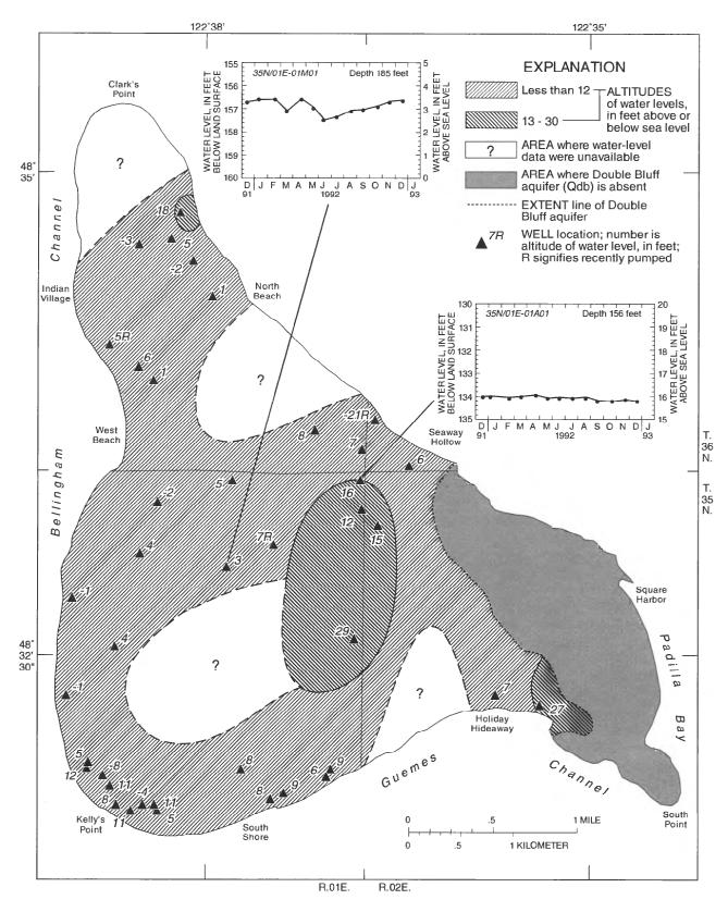
Figure 17.--Altitudes of water levels in wells completed in the Double Bluff aquifer (Qdb), and hydrographs of water levels in selected wells, October 1991.
