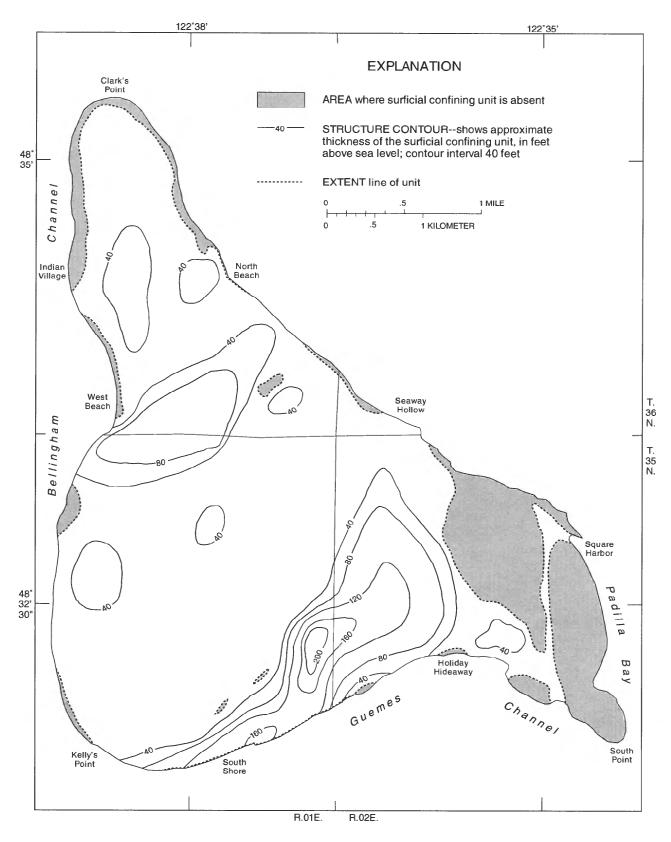
Figure 7.--Extent and thickness of the surficial confining unit.
