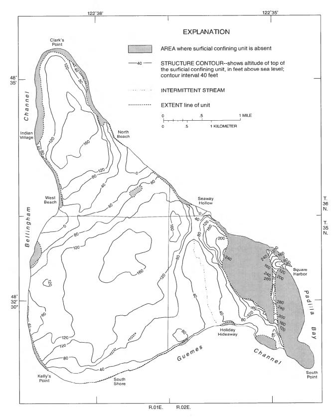
Figure 6.--Extent and altitude of the top of the surficial confining unit.
