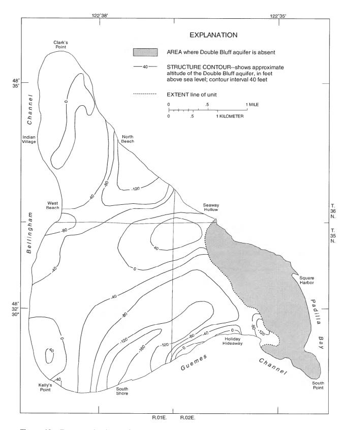
Figure 12.--Extent and altitude of the top of the Double Bluff aquifer.
