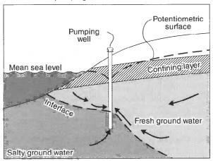
Figure 20.--Hypothetical hydrologic conditions (a) before and (b) after seawater intrusion (modified from Lum and Walters, 1976).
