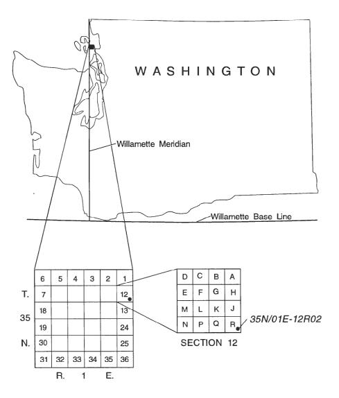
Figure 2.--Well- and spring-numbering system used in Washington.
