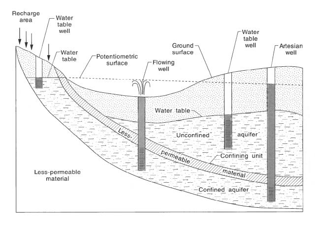
Figure 4.--Unconfined and confined ground-water conditions. (Modified from Todd, 1980.)
