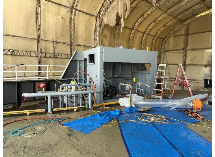
Engine Enclosure No. 1 with first coat of epoxy primer.
