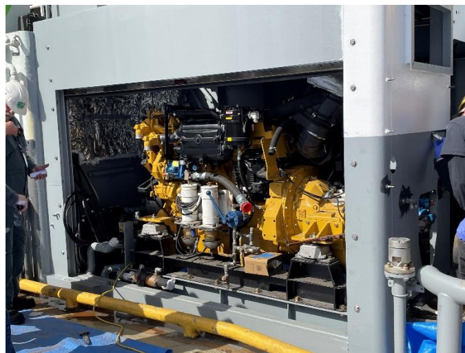
Engine No. 2 bolted to the new foundation.
