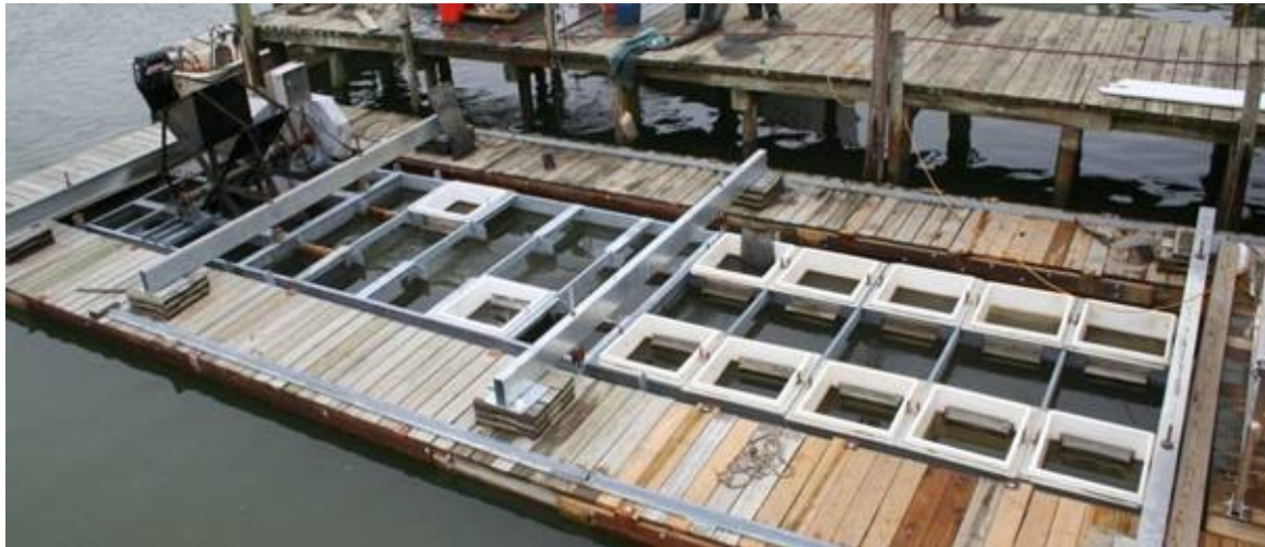
Figure 2: Floating Upweller System (FLUPSY) for raising oyster seed. (Photo source: Keri Weaver, City of Poulsbo)
