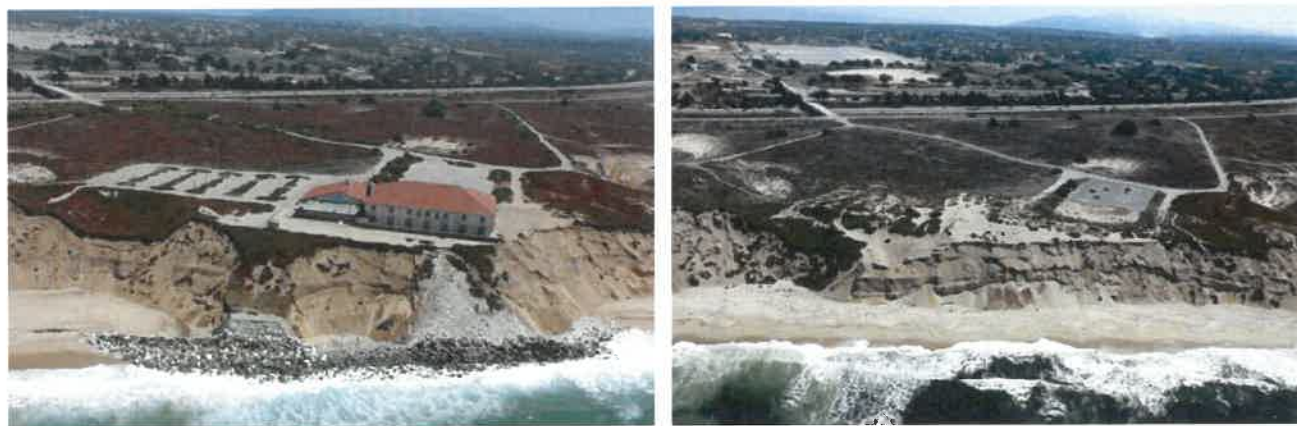
FIGURE 6.6 (Left) Passive erosion in front of a revetment, illustrating the loss of beach where the structure restricts the shoreline from migrating landward. The beach continues to migrate inland on either side of the revetment. (Right) Recovery of the beach following removal of the revetment and bluff top structure. SOURCE: Copyright 2002–2012 Kenneth & Gabrielle Adelman, California Coastal Records Project, < www.Californiacoastline.org >.
