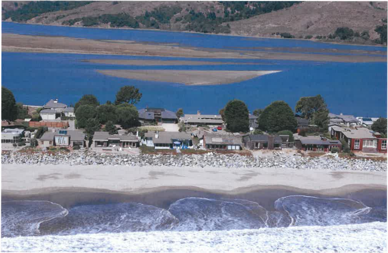
FIGURE 6.7 Developed sand spit at Stinson Beach in Marin County, California, where a revetment has been constructed in an effort to protect the homes. This spit cannot migrate with sea-level rise. SOURCE: Copyright 2002–2012 Kenneth & Gabrielle Adelman, California Coastal Records Project, < www.Californiacoastline.org >.
