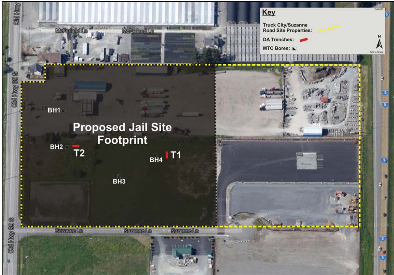
Figure 6. The Truck City/Suzanne Lane site with subsurface test units illustrated.
