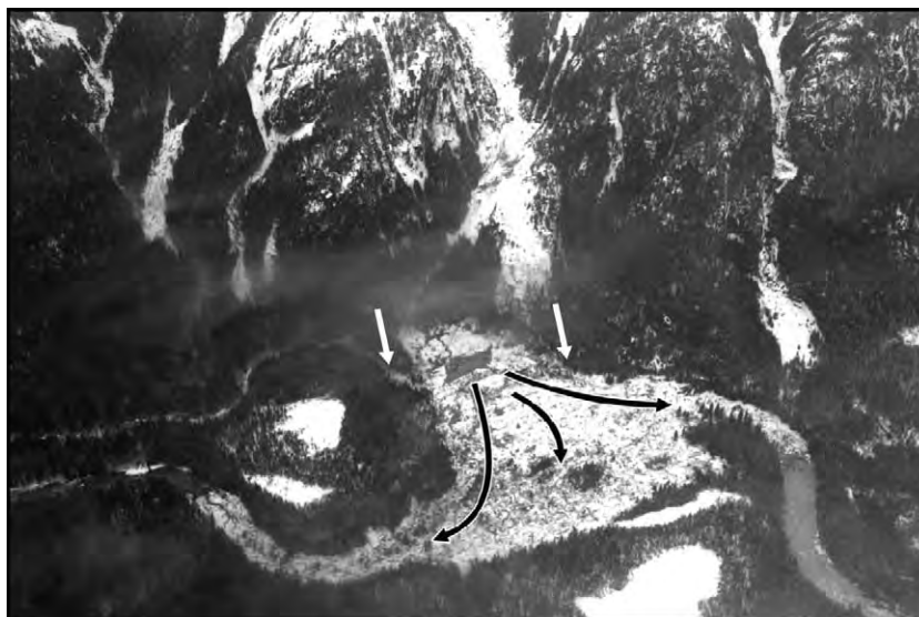
Fig. 14. The 2003 Khyex River earthflow in glacial marine sediments. The landslide ruptured a natural gas pipeline (white arrows), disrupting service to the city of Prince Rupert for about 10 days. Note the type III landslide dam, created where material flowed up and down river. Photo courtesy Prince Rupert Royal Canadian Mounted Police.
