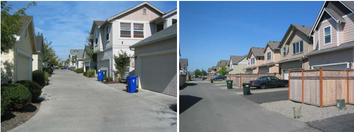
Figure 14.46.450(3). Desirable and undesirable alley designs. In the left image, landscaping elements between the fences and the alley enhance the appearance of the alley. Similar landscaping would help the example on the right.
