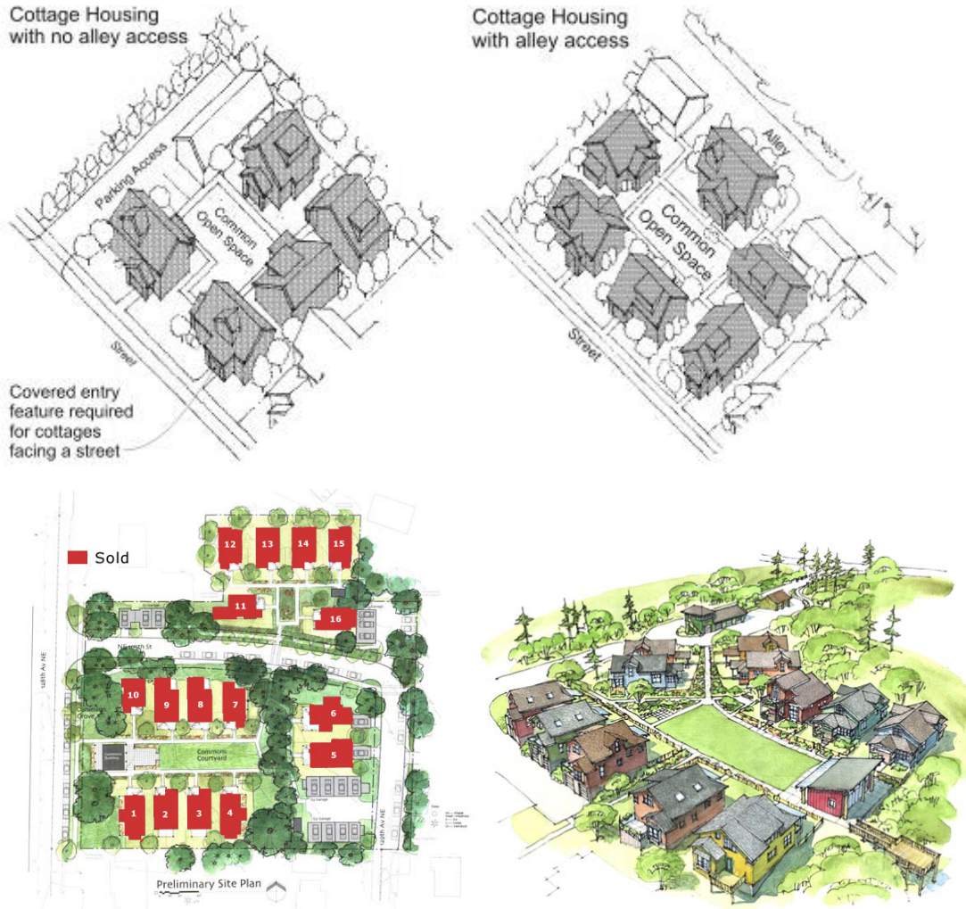
Figure 14.46.514(a). Typical cottage housing layouts.
