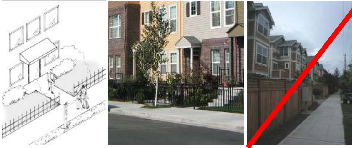
Figure 14.46.550(3)(a)(i). Acceptable and unacceptable fencing examples along a street.
