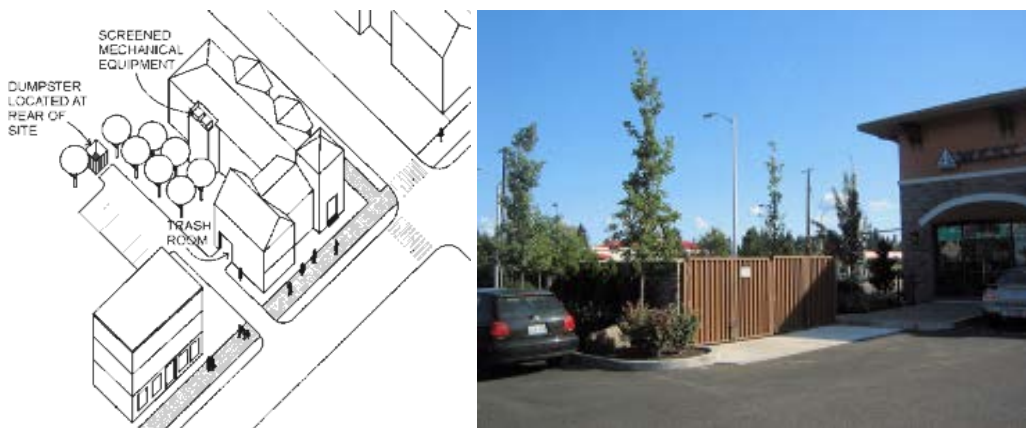
Figure 14.46.526(a). Appropriate service area location and enclosure example.
