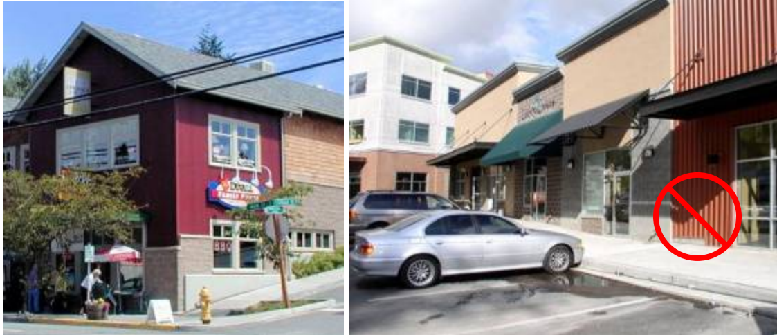
Figure 14.46.536(a). Acceptable and unacceptable metal siding examples. Notice the corner and window trim and use of concrete block near the ground level on the left image. The circled area on the right includes metal siding all the way to the ground, which is prohibited.
