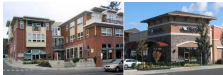
Figure 14.46.530(5)(a). Façade details examples. The building on the left uses decorative windows and doors, decorative roofline and columns, and decorative materials (brick and wood). The center image uses a decorative entry feature (metal feature over entry), decorative weather protection and lighting, and decorative use of brickwork. The right image uses decorative wood beams over the entry, decorative windows and doors, and stonework.
