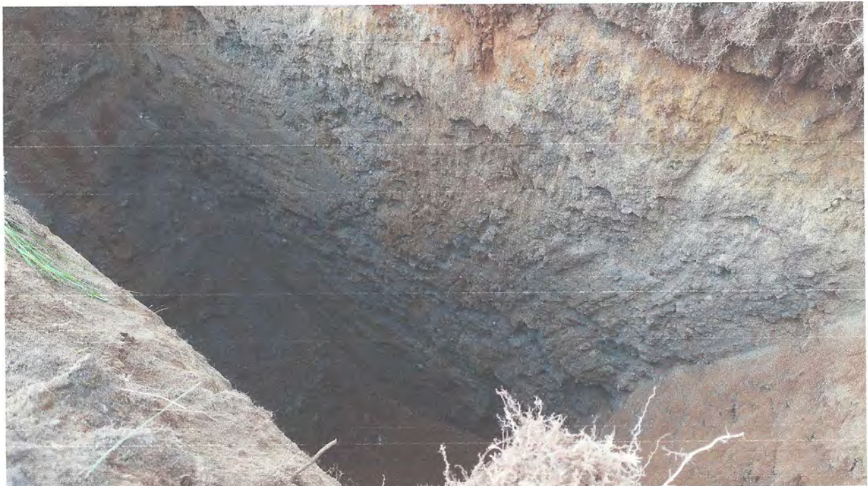
View of Test Pit 2 showing silt/clay glacial drift throughout test pit
