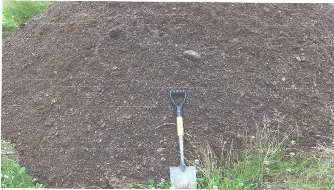
Coarse Sand with cobbles in test pit spoils from Test Pit 4
