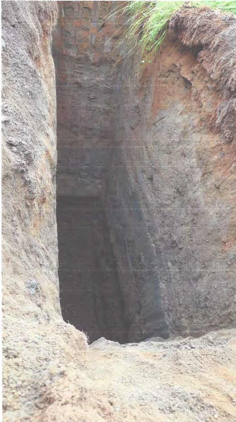
Test Pit 6 with silt and clay to 10 feet and gravel coarse sand and gravel below
