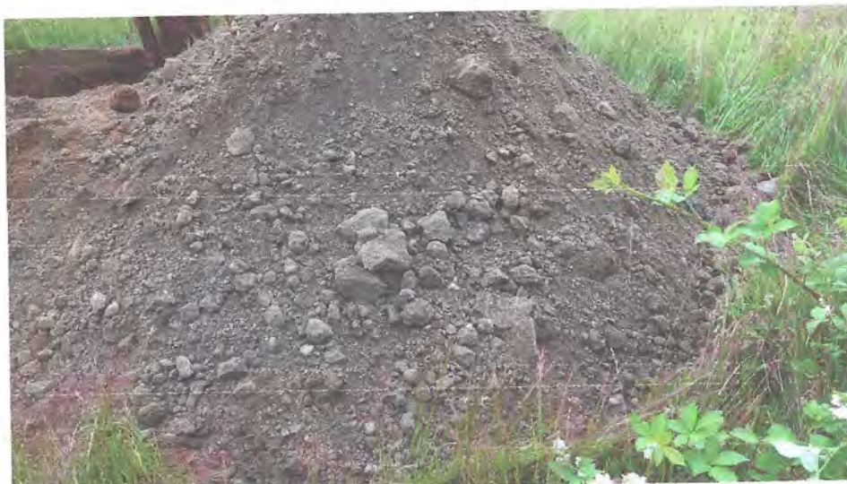
Blocks of silt/clay drift in test pit spoils on subject property
