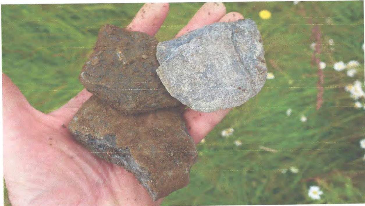
Typical rocks in alluvial fan sediment in upper part of Test Pit 5
