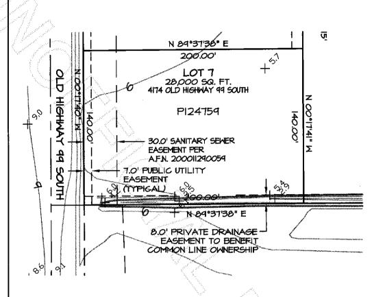
VERTICAL DATUM - N.G.V.D. 29 BASED ON A 6PS TIE MADE TO N.G.S. BENCHMARK DESIGNATION 6 331, PID TROOP, LOCATED 350 FEET WEST OF THE WEST QUARTER OF SEC. 32, TOWNSHIP 34 NORTH, RANGE 6 EAST, W.M., ELEVATION II.14 FEET N.G.V.D. 29.
